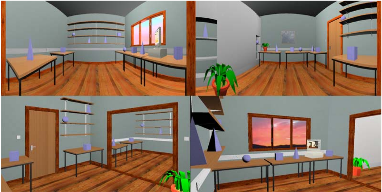
Flat Shaded version (top) Radiosity Rendered Version (bottom)
