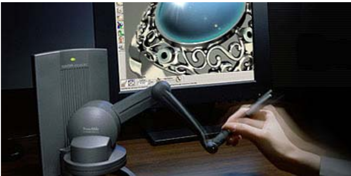
Figure 2.2: The application a tactile interface for product visualisation. With the stylus the user can 'feel' their way around a virtual object.
